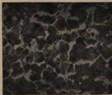
NO. 64. STRUCTURE \frac{1}{2} IN. BELOW TREAD.
